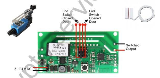
The limit switches (stops) for detecting open / closed doors can be, for example, a limit switch or a magnetic switch. For proper detection, the limit switches on the listed Sonoff SV terminals must make a closed circuit.
